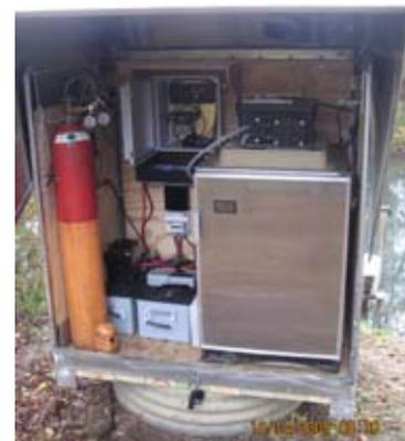
*USGS gaging station showing automated water-quality sampler and monitoring equipment.*
